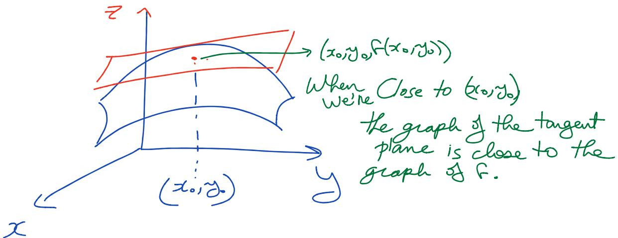
$$\text{Two variables: } z = f(x_0, y_0) + \left[ \frac{\partial f}{\partial x}(x_0, y_0) \right] (x - x_0) + \left[ \frac{\partial f}{\partial y}(x_0, y_0) \right] (y - y_0)$$
